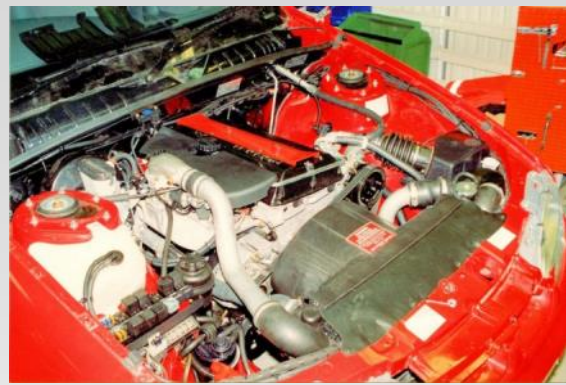
The Holden North-South Installation.
